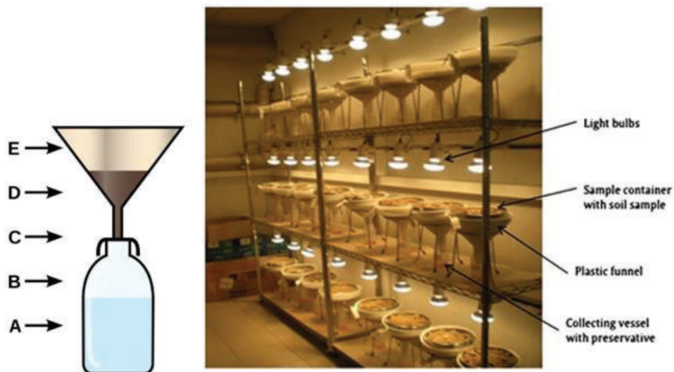
Example of a Berlese-Tullgren extractor (light bulbs are not required).
