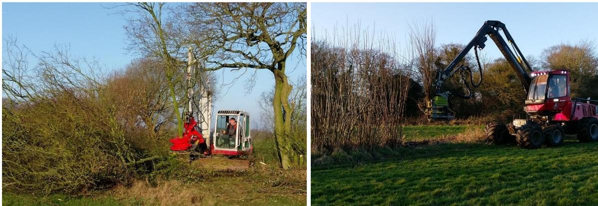
**Figure 16. (a: left) Tree shears harvesting mixed species boundary hedge (b: right) Bracke felling head in action on the SRC**
