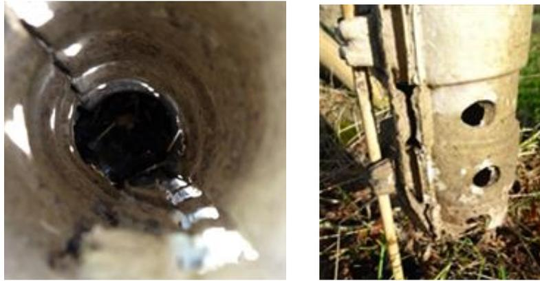
FIGURE 13. (LEFT) LIGHT CONDITIONS WITHIN THE BIODEGRADABLE FIBRE GUARD (RIGHT) DEGRADATION OF THE BASE OF THE BIODEGRADABLE FIBRE GUARD DUE TO WET WEATHER.
