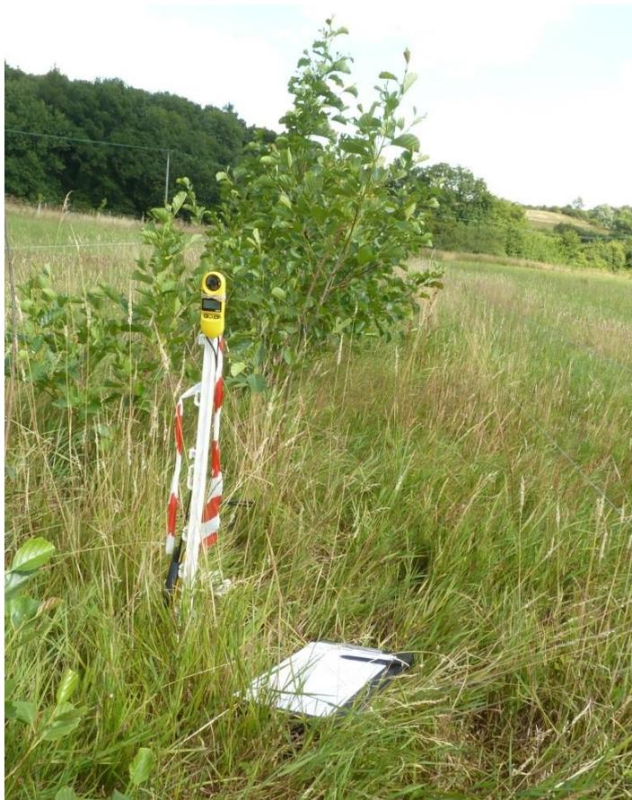
FIGURE 73. ANEMOMETER MEASURING WIND SPEED, AIR TEMPERATURE, WIND CHILL AND RELATIVE HUMIDITY AT THE ALLEY EDGE
