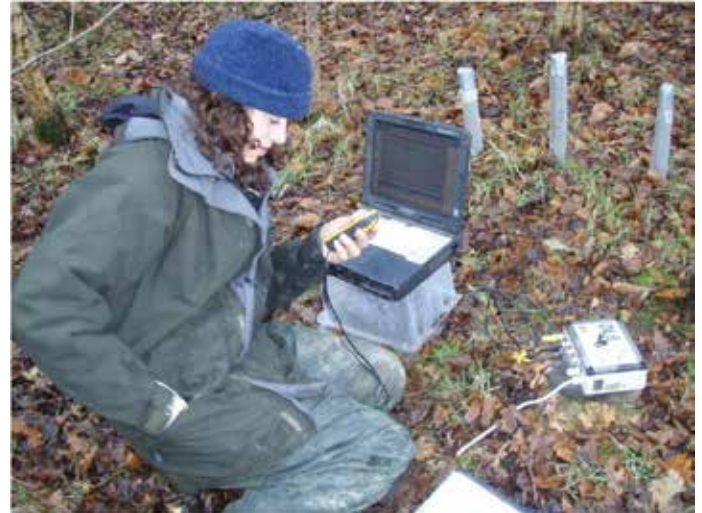
Infiltration rates inside the woodland were 60 times those on the pasture ten metres away. Photo: Coed Cymru.
